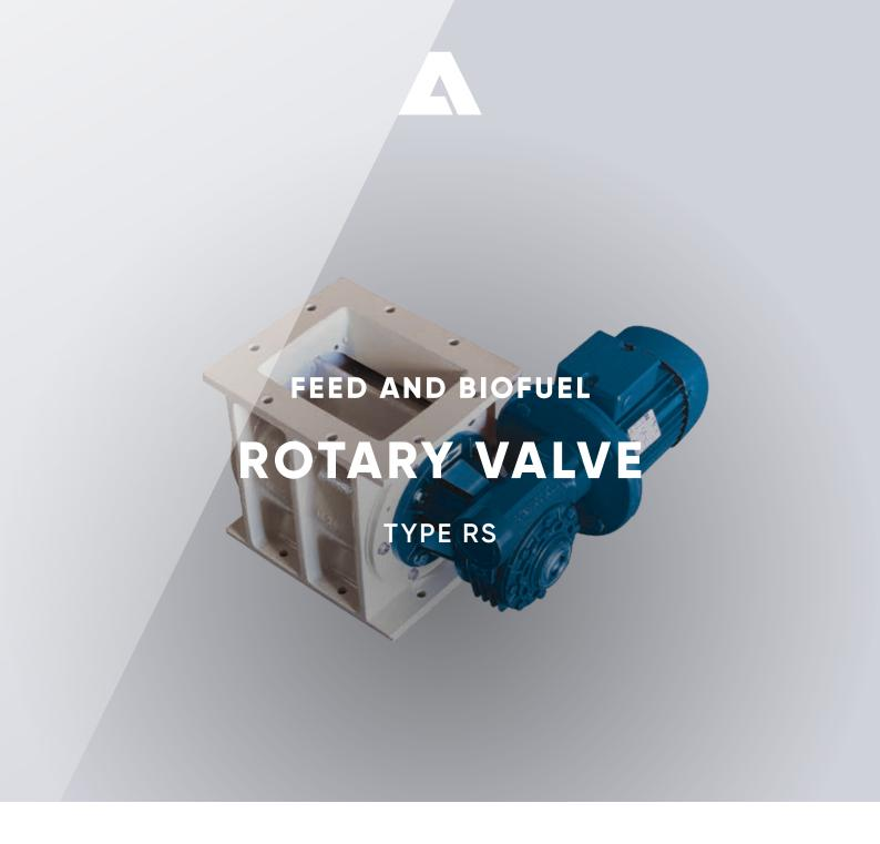
The rotary valve is used for continuous discharge of granular and powdered materials, for example from filters and cyclones. The RS type rotary valve is a compact unit with direct-mounted hollow shaft gear and motor. The housing and end covers are made of cast iron, and the rotor is welded in steel.
