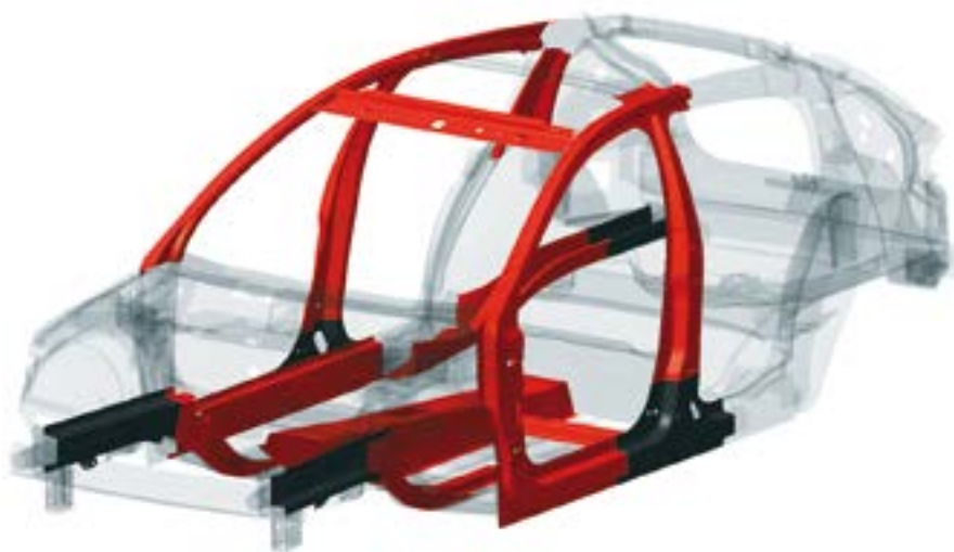
In order to enhance safety, press-hardened components are used in car bodies: softer components to absorb the impact energy (black) and rigid components for a stable passenger compartment (red). Photo: ArcelorMittal
