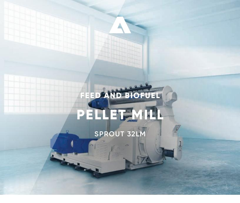
The ANDRITZ 32LM, with the most rugged design available is a 500 HP follow-up to the 26LM II with same quality and performance, just in a bigger scale.
