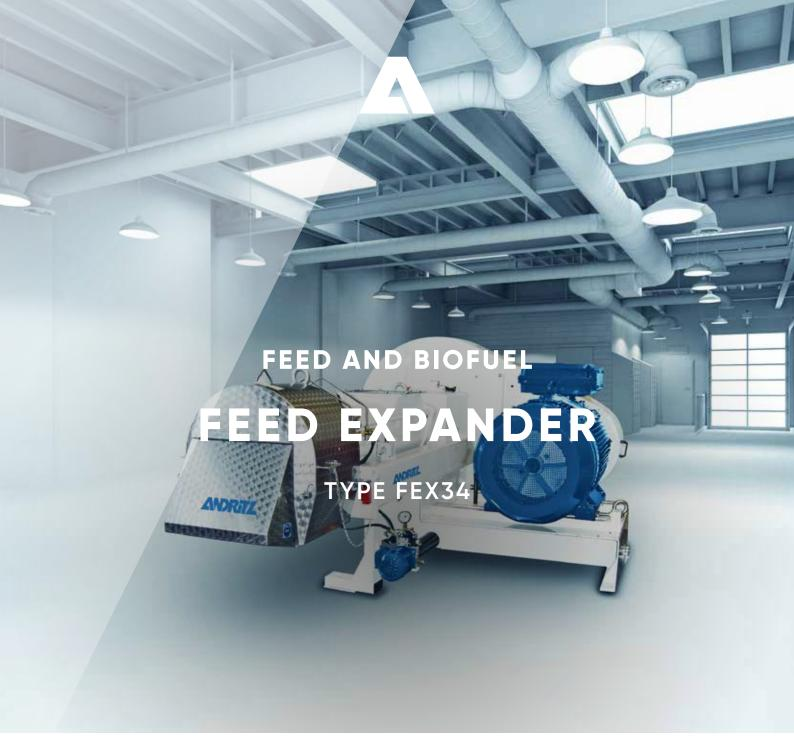
The feed expander is used to compress and heat the meal material prior to its compaction in a pellet mill. The expander consists of a barrel with a screw that kneads and conveys the material to the expander outlet. The expander outlet is provided with a cone, so that the material can be pushed through a gap.
